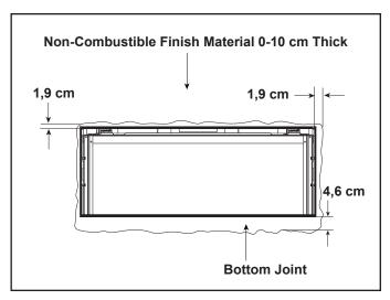
Figure 13.9 Noncombustible Surface Finishing Material 0 - 10 cm Thick-Inside Fit Method (Tonic Decorative Front Only)
